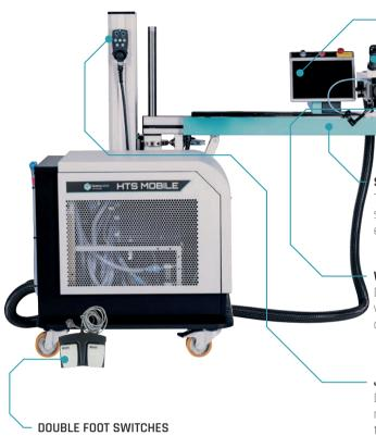
Enables two welding modes (single or continuous) with automatic shielding gas supply function.
